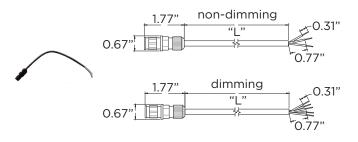
**OGLxxJxP - Jumper Cables** interconnects fixtures (xx) 12"-48" jumper lengths and either (x) 3 pins for non-dimming or 5 pins for dimming.
