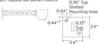
**Ax - Extended Arm** is an adder for swivel mounts. 4"-18" lengths. Fixtures 2ft+ require two arms.
