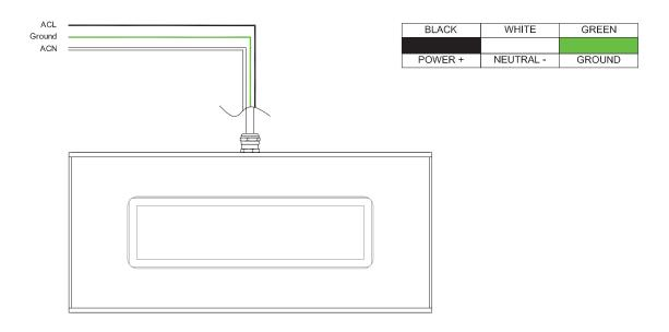
0-10V Dimming | 5 Wire | 120-277V
