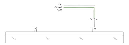
0-10V Dimming | 5 Wire |120-277V
